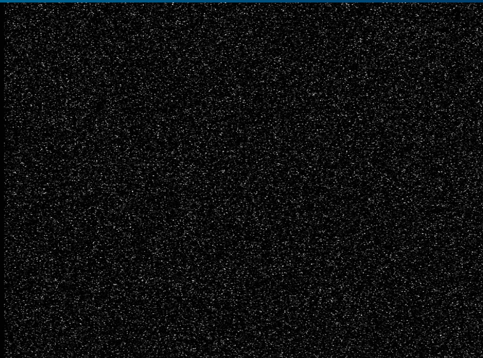
b) CCD after use on fast neutron source “Noise” much greater than specifications
